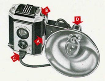
Install the Batteries by lifting either one of the metal clips on the back of the Flasholder battery case and removing the back cover. Place two pen-sized pocket flashlight batteries in the case so that their heads point in opposite
