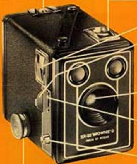
**CATCH** . . . Lift to open camera for loading and unloading film
